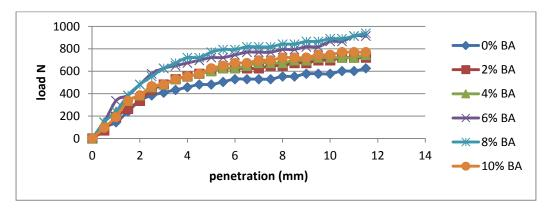
Fig. 3. CBR plot for soil with bagasse ash and single layer geogrid
