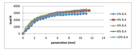
Fig. 2. CBR plot for soil with bagasse ash
