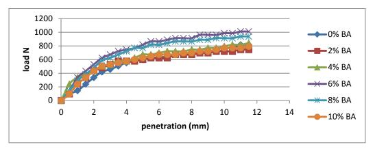
Fig. 4. CBR plot for soil with bagasse ash and double layer geogrid
