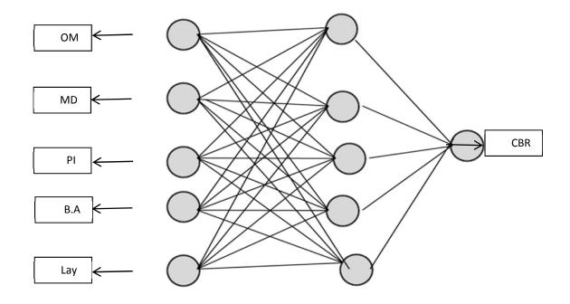
Fig.10. Architecture of Neural Network model
