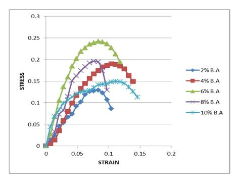
Fig.7. Comparison UCC graph for soil with bagasse ash
