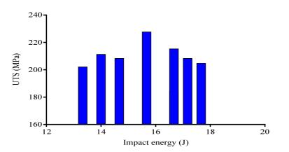
Figure 9 Bar charts of UTS against impact energies at ageing temperature of 170 °C (Al-Si-Mg alloys)
