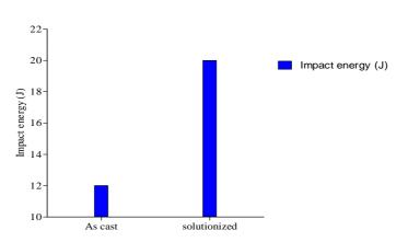
Figure 6 Impact energy of as-cast and solution treated sample
