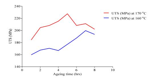
Figure 3 Composite curves for Al-14%Si-0.288Mg at 160 °C and 170 °C for 8 hours
