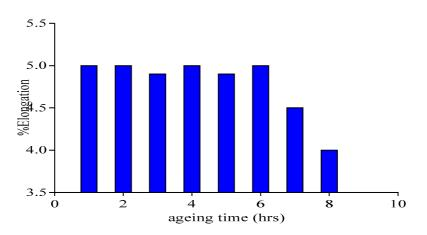
Figure 4 Effects of ageing time on the ductility of samples 160 °C
