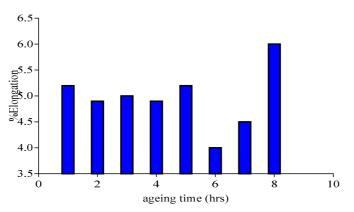
Figure 5 Effects of ageing time on the ductility of samples at 170  $^{\circ}$ C
