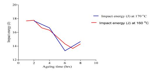
Figure 7 Composite curves of impact energies at 160 °C and 170 °C for Al-Si-Mg alloy
