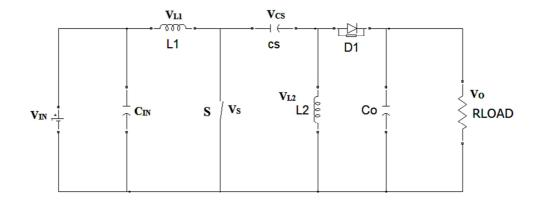
Fig. 1. Schematic diagram of conventional SEPIC converter
