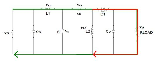
Fig. 3. Current flows during switch is turn off condition
