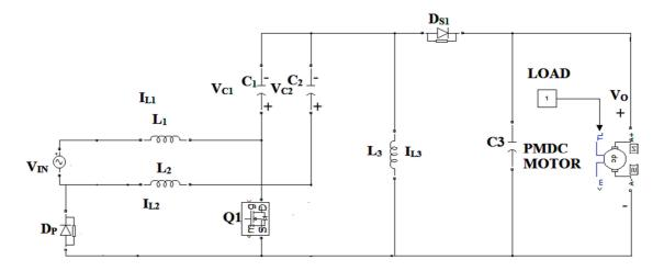
Fig. 8. During positive half cycle, switch  $Q_1$  turn on and  $Q_2$  turn off condition
