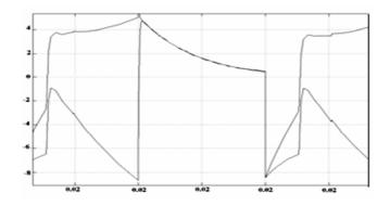
Fig. 15. Inductors  $L_1$  and  $L_2$  voltage waveforms
