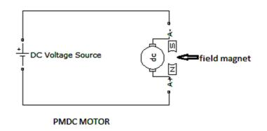
Fig. 4. Permanent magnet DC motor
