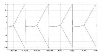
Fig. 14. Capacitors  $C_1$  and  $C_2$  voltage waveforms
