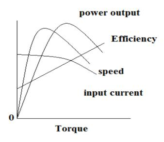
Fig. 6. Charteristics of PMDC motor
