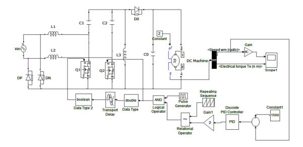
Fig. 7. Bridgeless SEPIC converter circuit diagram
