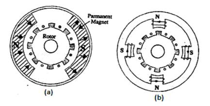
Fig. 5. Construction of permanent magnet in PMDC
