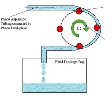
Combining these suction and discharge actions results in a self-priming positive displacement pump, the peristaltic pump.
