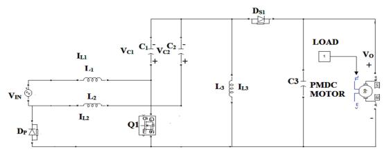
Fig. 10. During positive half cycle, switch  $Q_1$  turn on and  $Q_2$  turn off condition.
