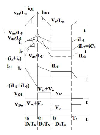
Fig. 12. Theoretical waveforms in DCM of proposed converter
