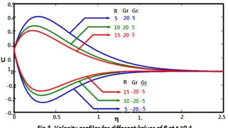
Fig.3. Velocity profiles for different values of R at t =0.4
