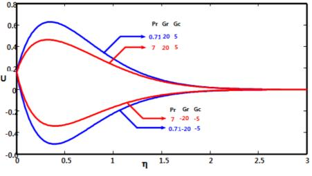
Fig.6. Velocity profiles for different values of Pr at t =0.4
