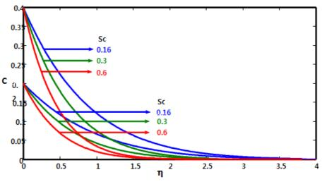
Fig.7. Concentration profiles for different values of Sc at t=0.2 and t=0.4
