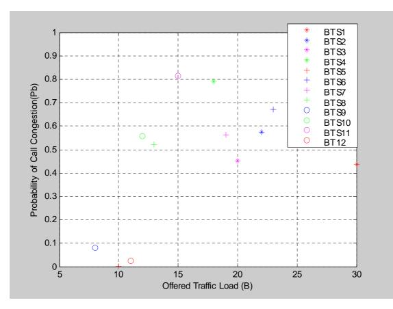
Fig.6 Graphical representation of the Simulation result for Fixed Channel Assignment Technique implemented on the 12 BTSs using assumed parameters values.
