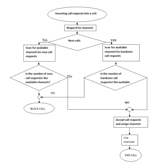
Fig 7 Flow diagram for the implementation of Fixed Channel Assignment Technique on a Congested Mobile Radio Network
