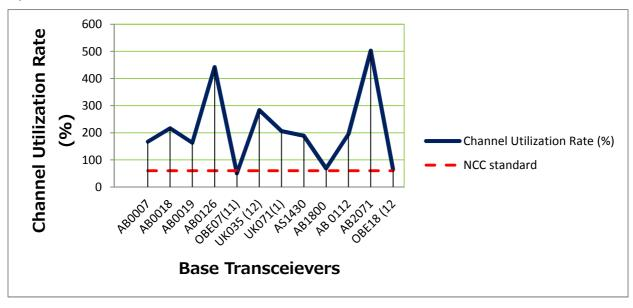
Fig 3 Comparing Channel Utilization Rate of the Network with the NCC Standard
