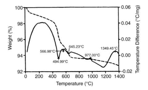
Figure 1: DTA Curve of Granitic Igneous Rock (Heitor 2001)
