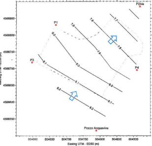
Fig.6. Groundwater flow direction below Andria Section A) landfill
