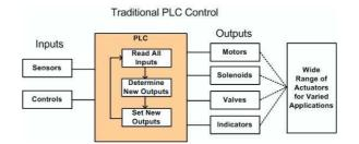
In this application, it controls through analog/digital inputs and outputs by varying the speed through VFD of an induction motor. Also the PLC reads the input and control the outputs according to the PLC program. This PLC is a Delta type of ISP software where the link is made to the system through RS232 cable. It has an advantage that the initial configuration can be expanded for the other applications as machine systems and computer related linking
