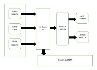
Fig.1 Block Diagram Representation of the System
