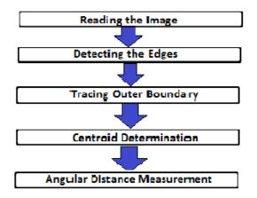
Fig.1. Feature Extraction Flow Diagram
