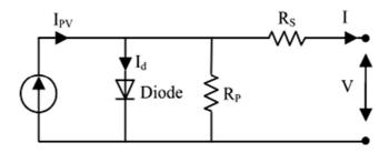
Figure 2. Equivalent Cricuit of pv cell
