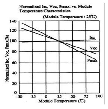
Figure 6. Typical PV Module Temperature Performance
