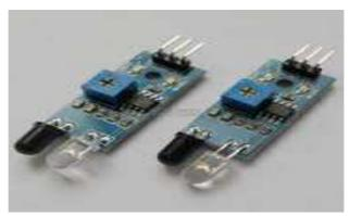
Figure: 4 Pictorial Representation Of Infrared-Sensor
