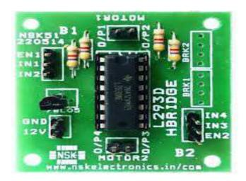
Figure: 10 H Bridge with different ports
