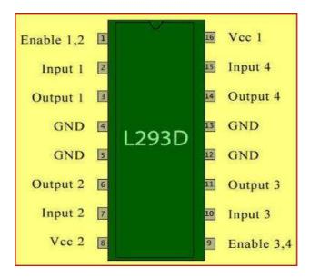
Figure: 11 L293D IC Pin Configuration
