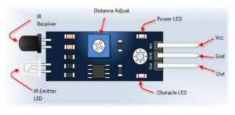
Figure: 5 Functional Pin Diagram of IR Sensor
