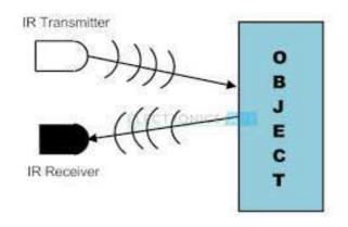
Figure: 6 Functional Representation of IR Sensor
