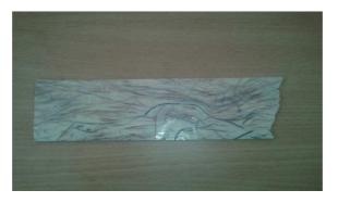
Fig 3.15 Final composite for tensile testing
