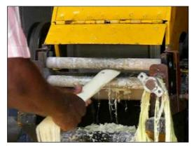
Fig.3.3 Banana fibre extraction machine
