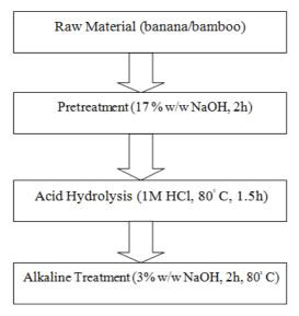
Fig 3.13 Process of chemical treatment
