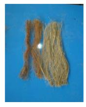
Fig. 3.10 Bamboo and Banana Fibres
