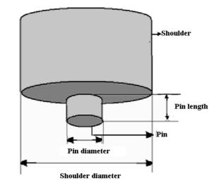
Figure 4: Tool Geometry
