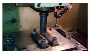
Fig.1. Friction Stir Welding Experimental Setup
