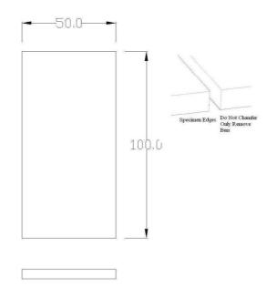
Figure 2: Workpiece Dimensions
