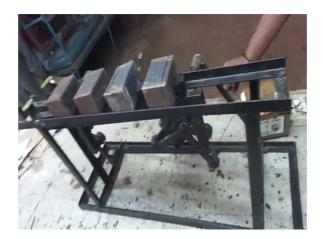
Fig.2.1 Four bar linkage
