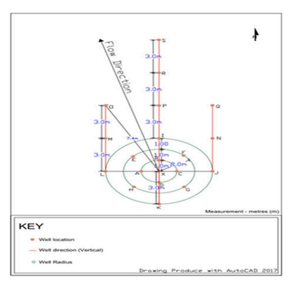
Fig. 1. Schematic Layout of tracer test field design
