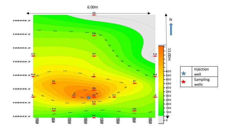
Fig. 2. Avector and concentration map illustrating the mignitude and direction of tracer within the tracer test site
