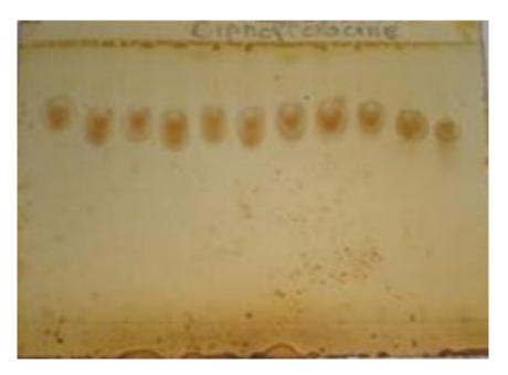
Fig. 2. TLC plate photograph of ciprofloxacin samples
