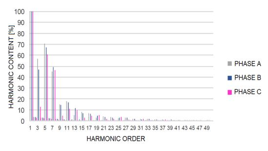
Fig. 5. FC110307T4OYZ current harmonic spectrum
