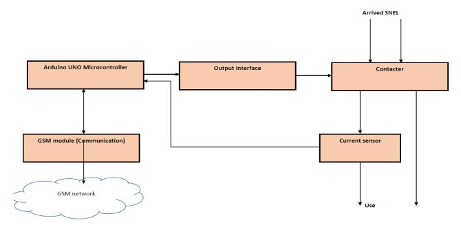
Fig. 2. Block diagram of the sampling system
