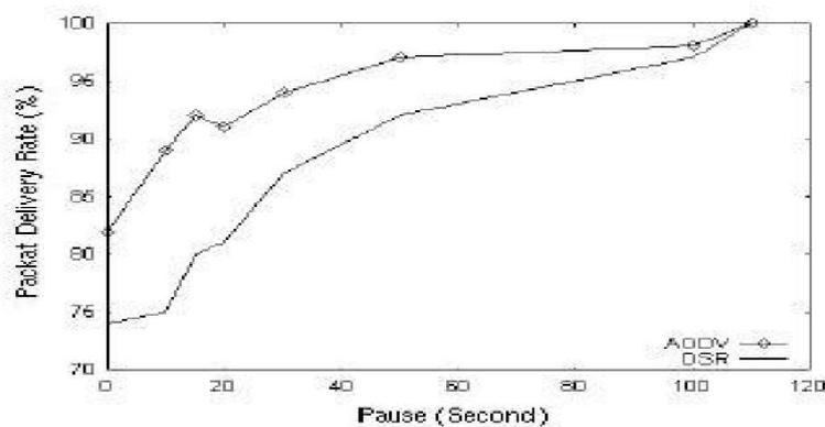
Fig. 4. Packet Delivery Rate vs. Pause Time
