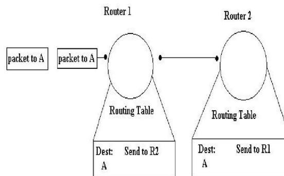
Fig. 2. The routing process from source to destination
