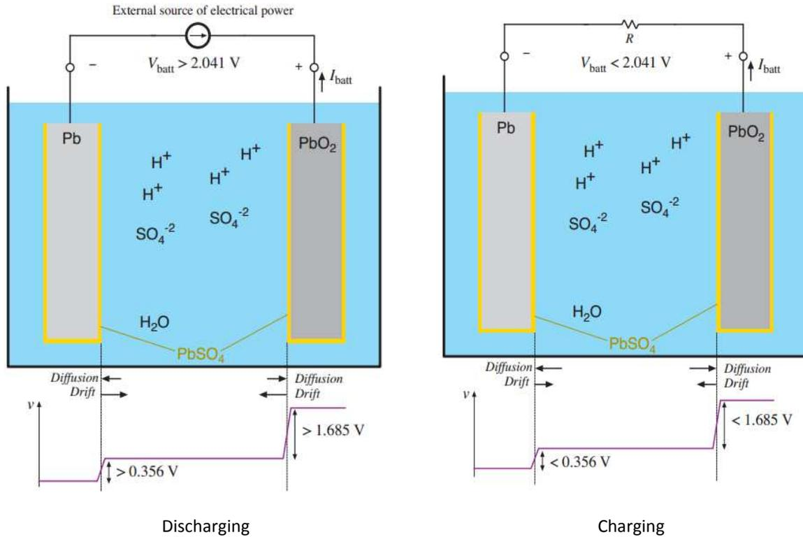
Fig. 2. Charging and discharging of lead-acid battery [17]
