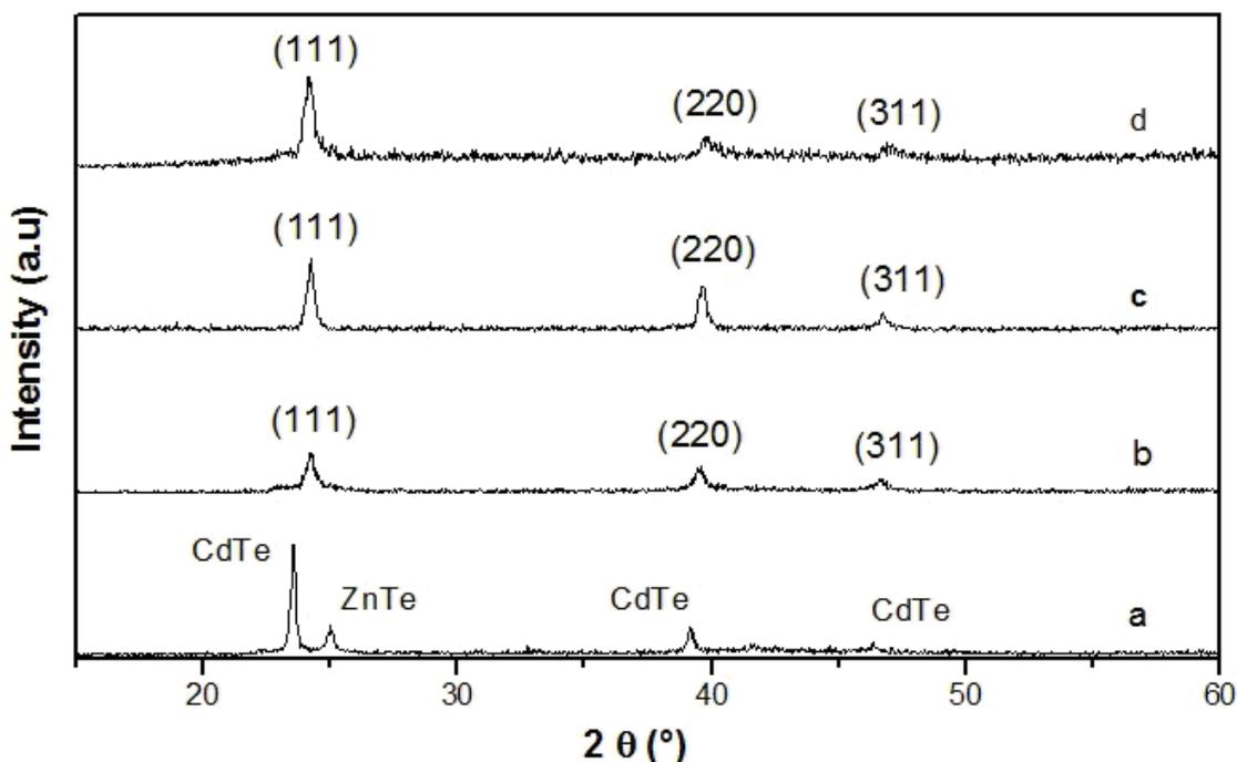
Fig.1. XRD patterns of: (a) as-deposited films; (b-d) annealed at 300; 350 and 400 °C respectively for 2 hours.
