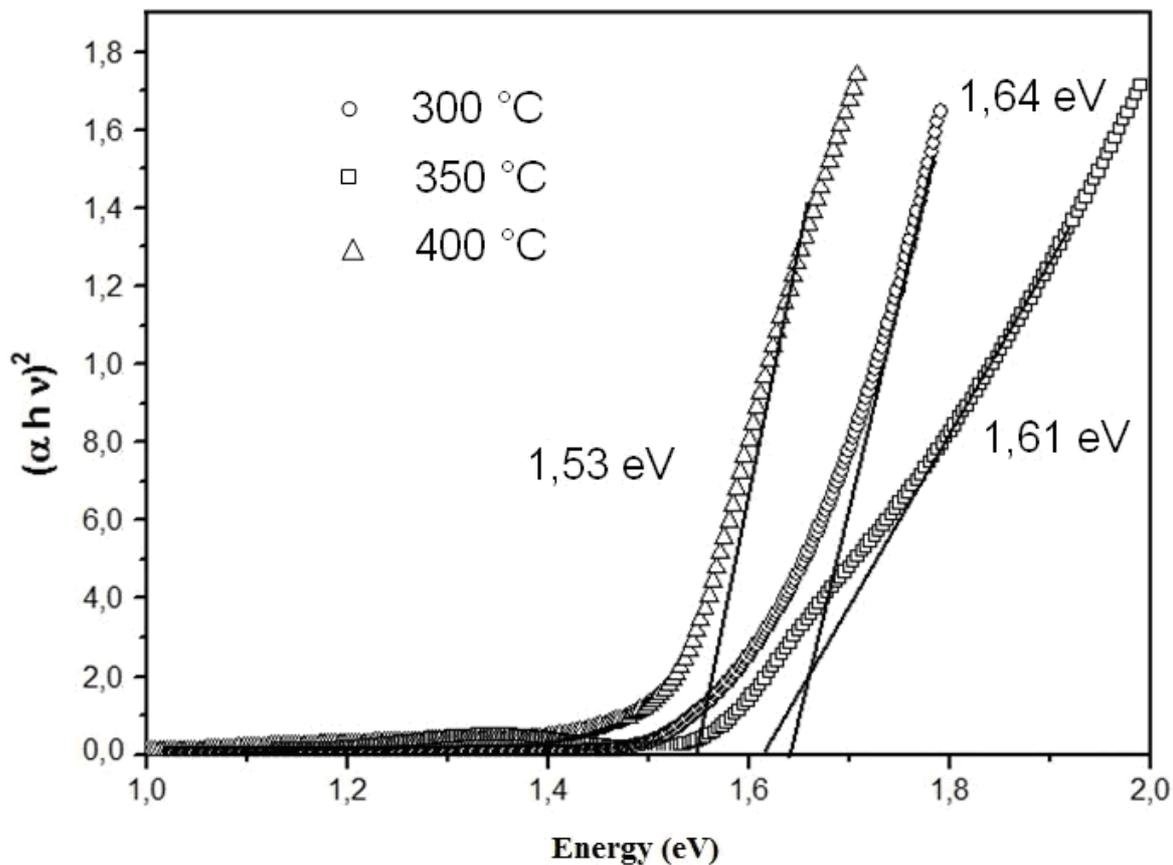
Fig.3. Variation of  $(\alpha h\nu)^2$  as a function of photon energy ( $h\nu$ ) for Cd<sub>1-x</sub>Zn<sub>x</sub>Te thin films annealed at different temperatures
