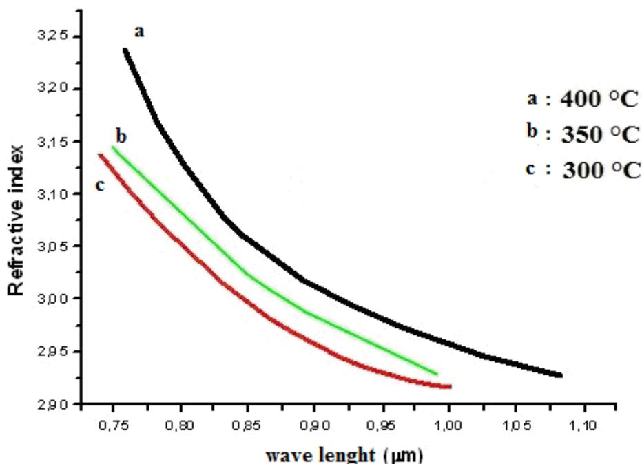
Fig.4. Variation of refractive index versus wavelength for Cd1-xZnxTe films annealed at different temperatures
