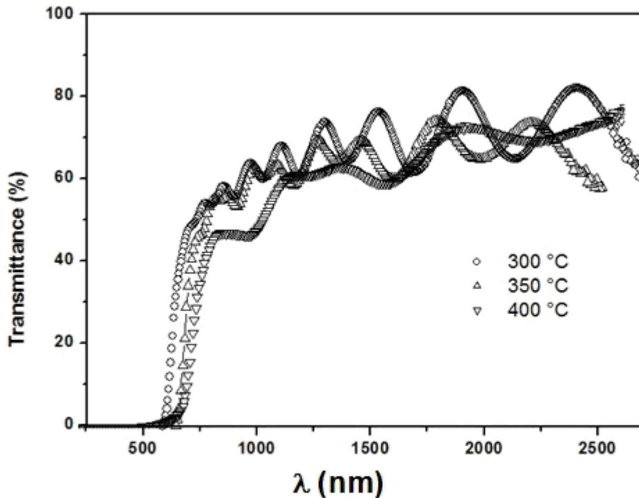
**Fig.2.** Normalized transmittance spectra of  $Cd_{1-x}Zn_xTe$  films annealed at different temperatures
