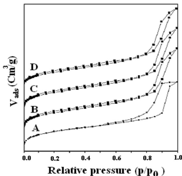
**Fig.1. N<sub>2</sub> adsorption-desorption isotherms of different Ni- SBA-15 catalysts. (A) 10Ni-SBA-15, (B) 30Ni-SBA-15, (C) 50Ni-SBA-15, (D) 70Ni-SBA-15**
