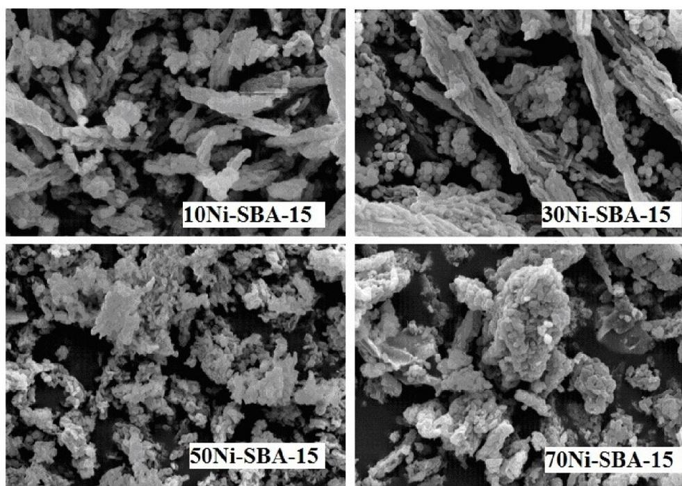
**Fig.4. SEM Images of different Ni- SBA-15 catalysts. (A) 10Ni-SBA-15, (B) 30Ni-SBA-15, (C) 50Ni-SBA-15, (D) 70Ni-SBA-15**
