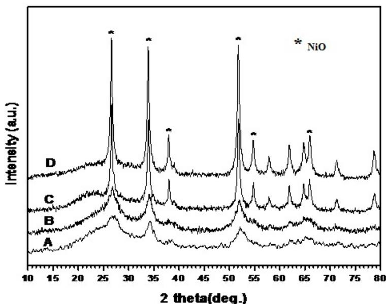
Fig.3. X-ray diffraction patterns of different Ni- SBA-15 catalysts. (A) 10Ni-SBA-15, (B) 30Ni-SBA-15, (C) 50Ni-SBA-15, (D) 70Ni-SBA-15
