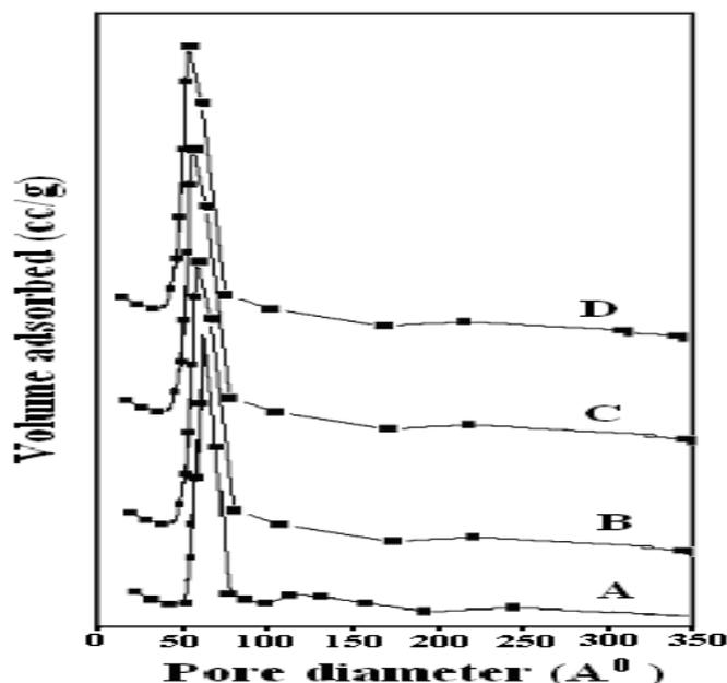
Fig.2. Pore size distribution of different Ni- SBA-15 catalysts. (A) 10Ni-SBA-15, (B) 30Ni-SBA-15, (C) 50Ni-SBA-15, (D) 70Ni-SBA-15
