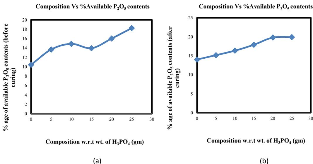
Figure-3: Relation between single super phosphate samples with % Available P<sub>2</sub>O<sub>5</sub> contents (a) Before curing (b) After curing
