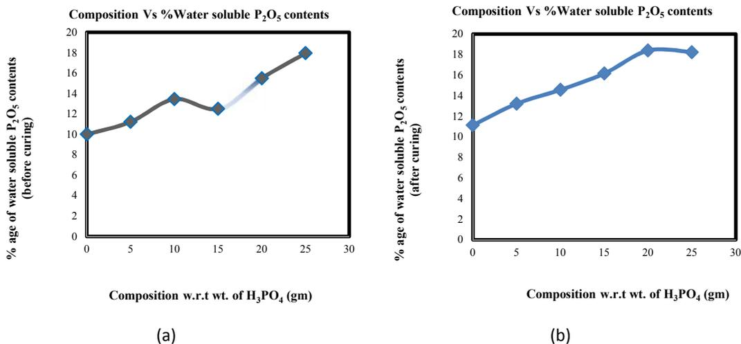
Figure-2: Relation between single super phosphate samples with % water soluble P<sub>2</sub>O<sub>5</sub> contents (a) Before curing (b) After curing
