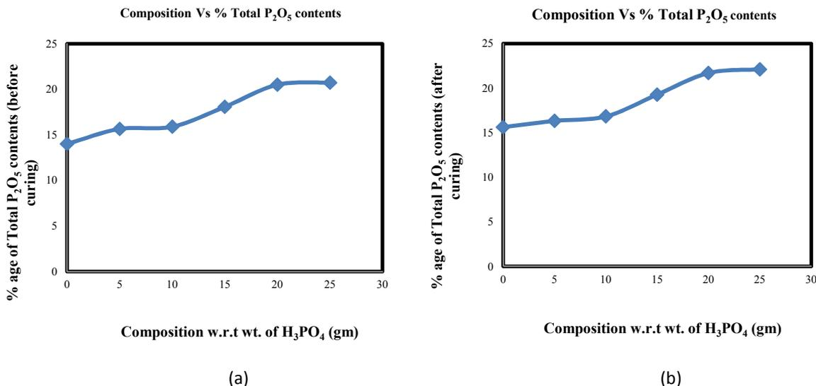
Figure-1: Relation between single super phosphate samples with % total P<sub>2</sub>O<sub>5</sub> contents (a) Before curing (b) After curing
