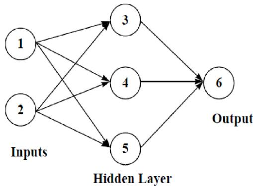
Fig. 4. Sample Artificial Neural Network
