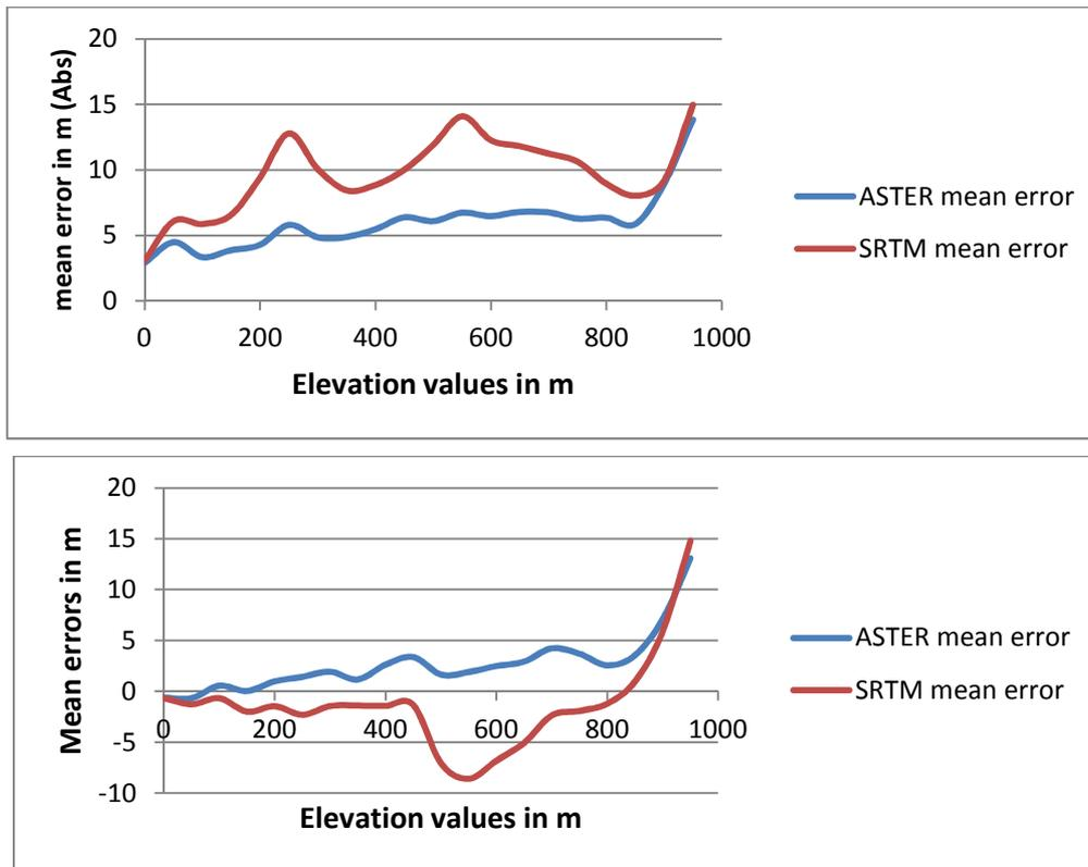
Fig. 6. Vertical accuracy of ASTER and SRTM relative to terrain morphology
