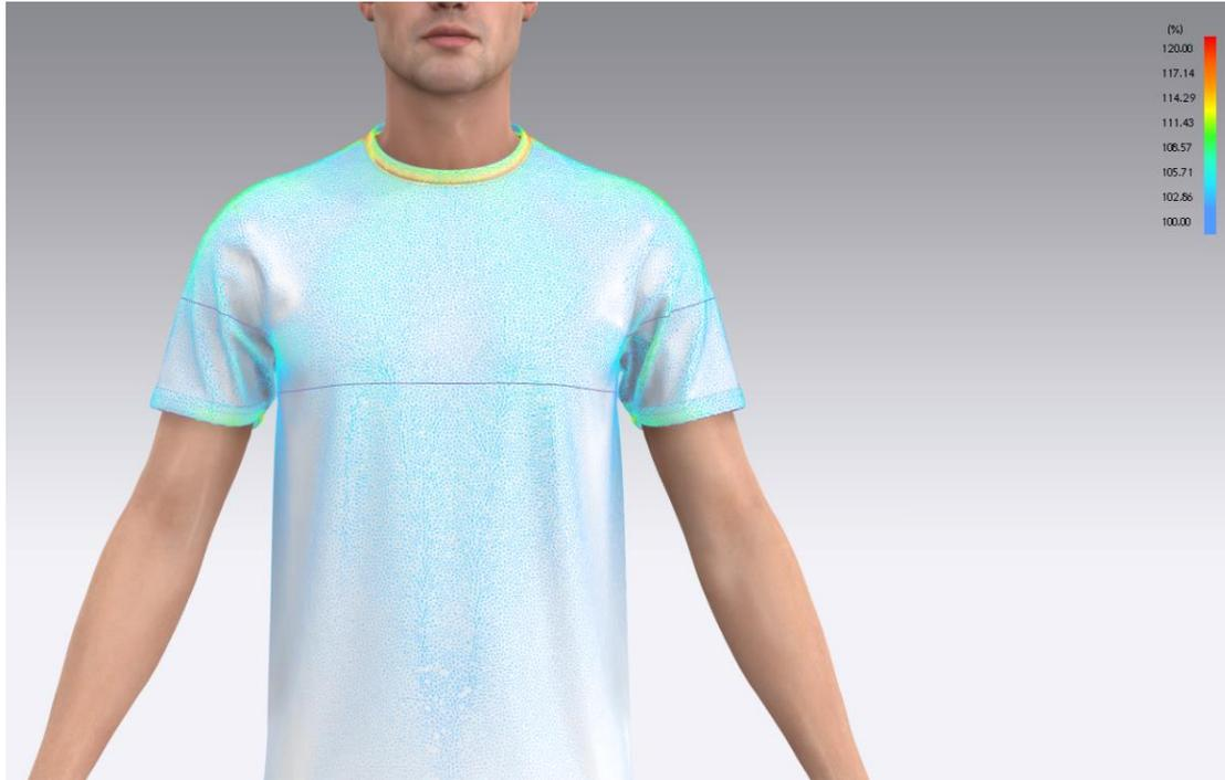
Fig. 5. Observed special feature for checking tightness or looseness in Lectra software
