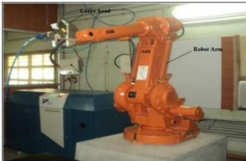
*Fig. 1. Laser beam welding unit*
