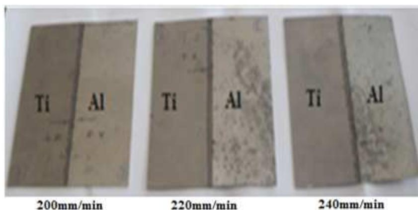
*Fig. 4(a). Macrostructure of welds on top side*
