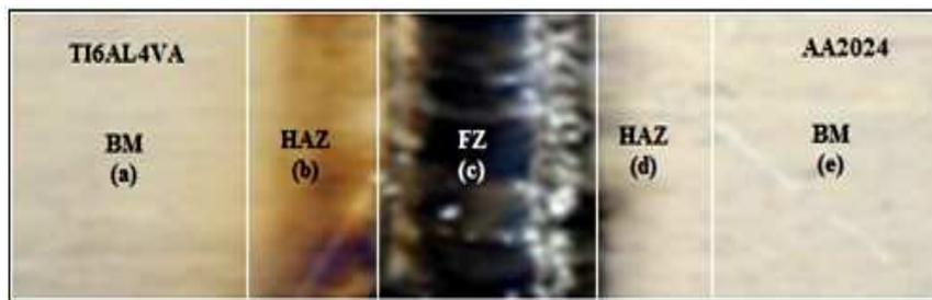
Fig. 5. Various zone at weldment both Ti/Al sides
