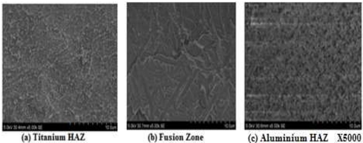
**Fig. 7. Microstructure at 220mm/min, laser beam focused from Ti side (a) Ti HAZ, (b) Fusion Zone and (c) Al HAZ**
