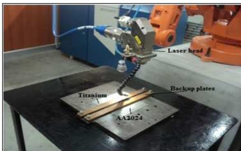
*Fig. 2. Clamping device with backup plates*
