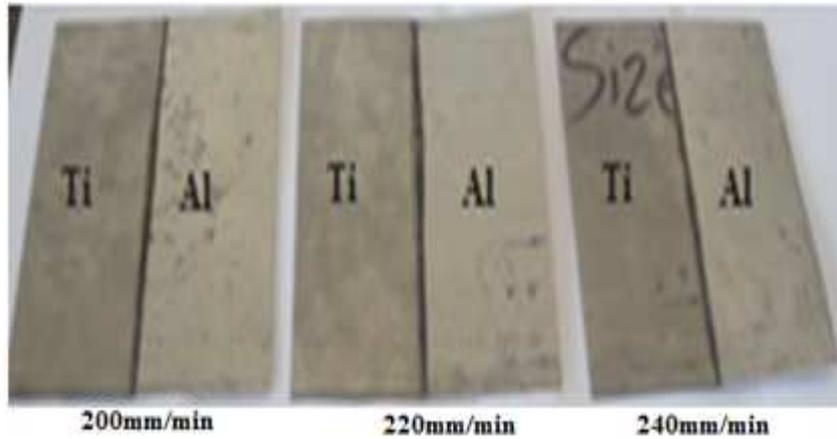
Fig. 4(b). Macrostructure of welds on bottom side
