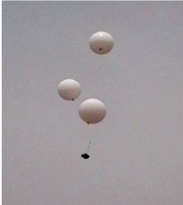
Fig. 2. Airborne System with three high altitude balloons for better lift
